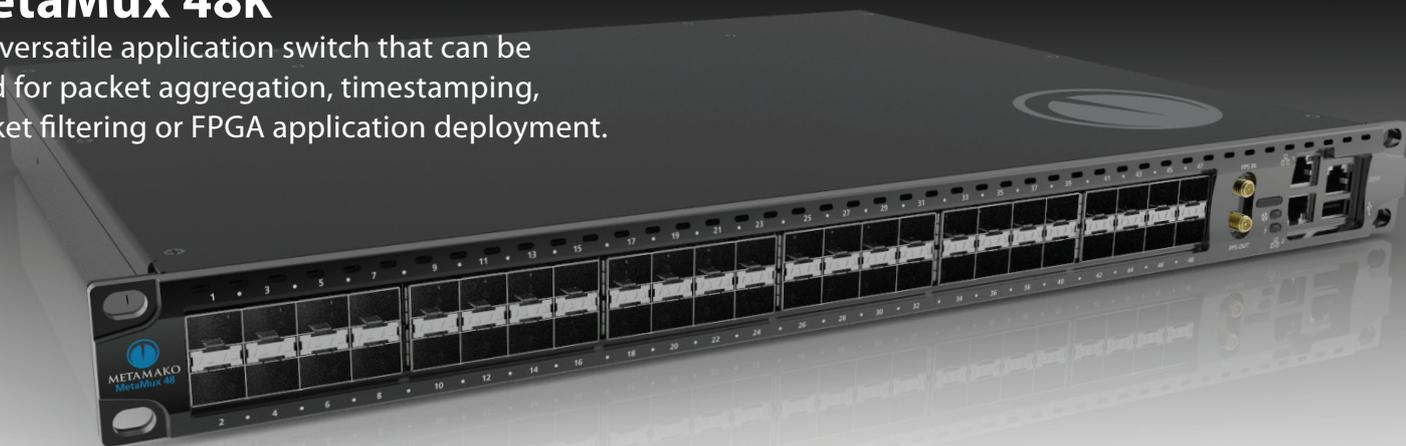
**MetaMux 48K** is a versatile application switch. MetaMux 48K is optimised to run MetaWatch, a tap-aggregation and high-resolution timestamping solution with deep buffering, but may also be configured to perform layer 1 switching in only 5 ns, multiplexing/aggregation in 99 ns or filtering at 95 ns. It has an on-board Xilinx Virtex 7 FPGA and can also be used as an application deployment platform
